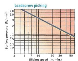
Pressure on and sliding speed of nut surfaces determine the appropriate leadscrew design.
